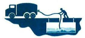
Many septic tank owners believe that if they haven't had any problems, they don't need to have their septic tanks pumped. If the solids are not removed, eventually they will flow out of the tank damaging the rest of the system. The following chart can be used as a guide to assist you as to when to have your tank pumped.
